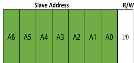
Fig.5 Standard I2C 7-bit addressing format
